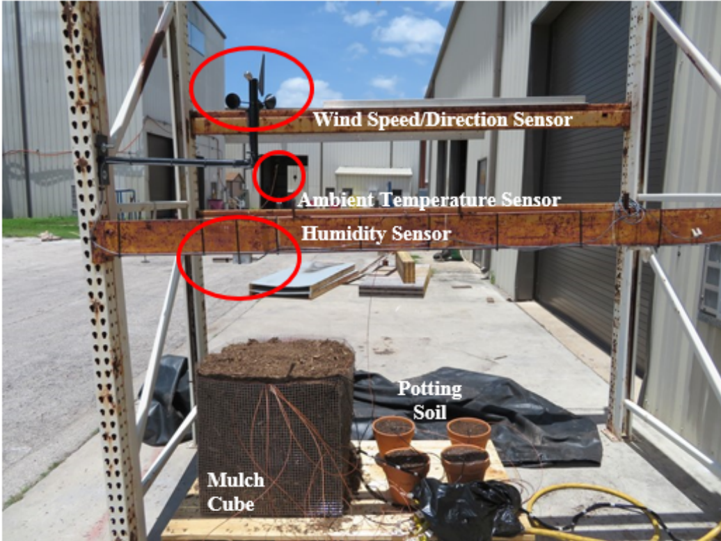
Figure 5. Intermediate-Scale Testing – Outdoor Setup (Ambient Sensor Locations Indicated).
